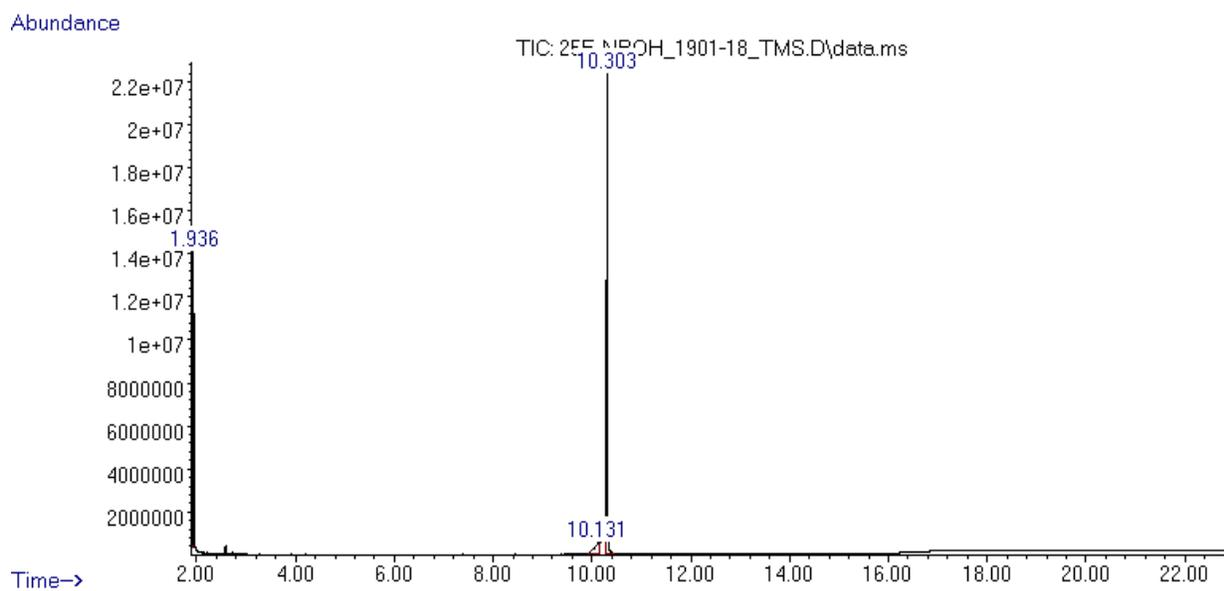
Chromatogram: mono-TMS derivative (O-TMS) at 10.13 and di-TMS derivative O,N-diTMS at 10.30 min.
