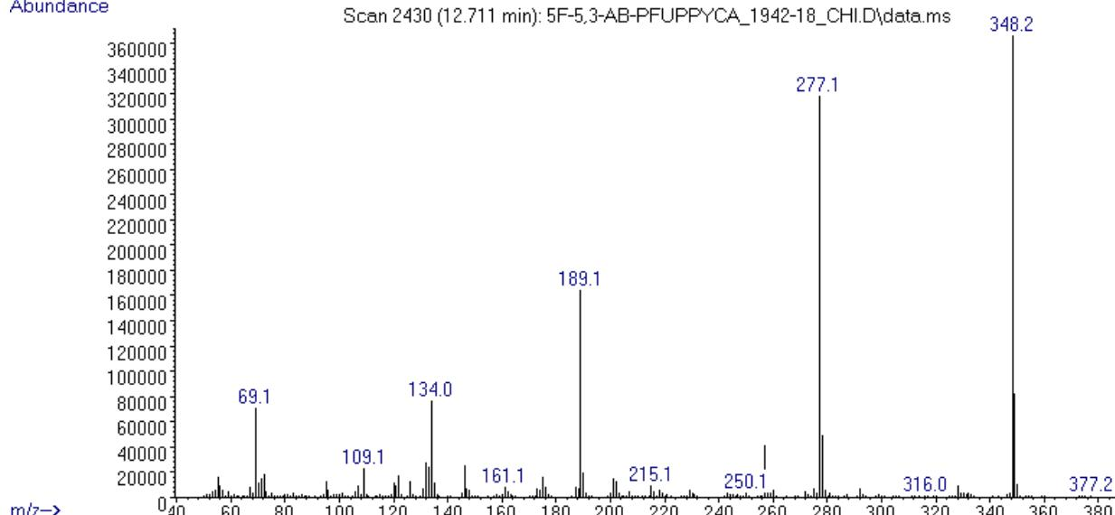
MS at peak apex (measured at split ratio 50:1)
