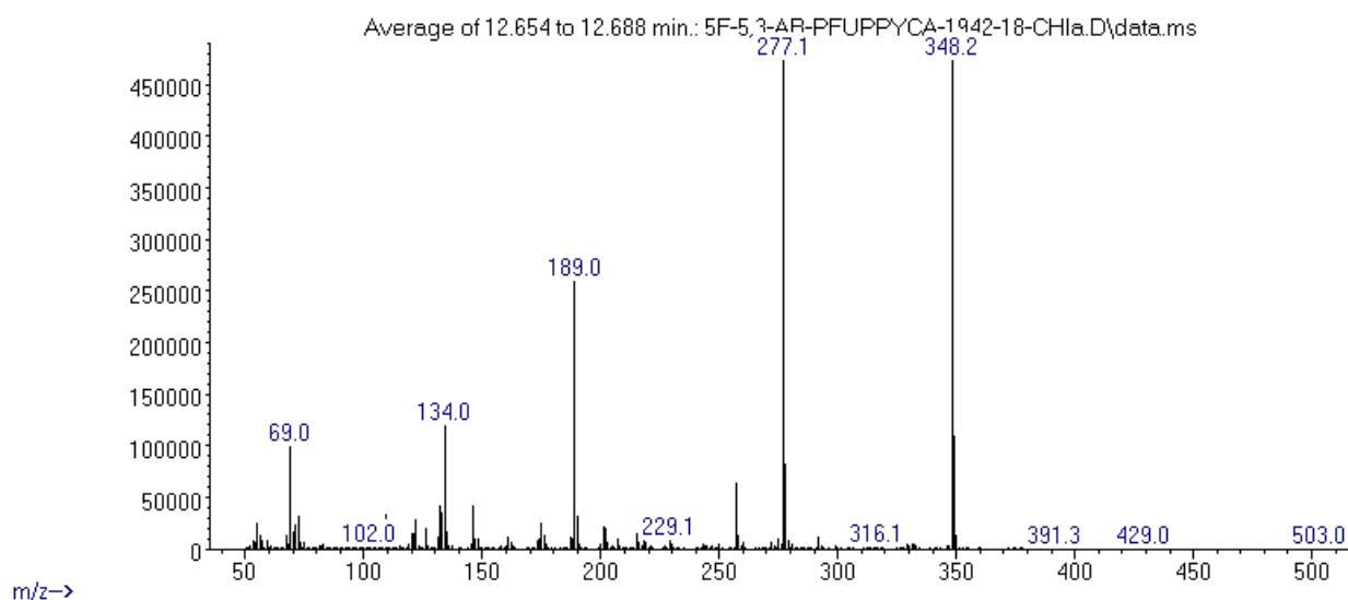
MS - averaged spectrum (measured at split ratio 25:1)
