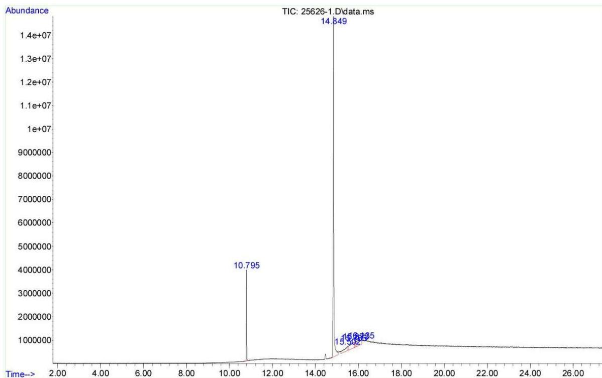
Agilent 6890N Network GC system set up with Agilent HP-5MS
