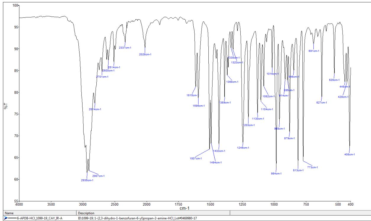
IR- (condensed (solid) phase – after chromatographic separation) - spectrum per base form
