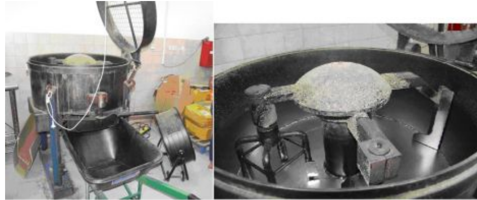
Mixing machine: raw plant material + synthetic cannabinoid dissolved in acetone is mixed until acetone is evaporated (some preparations can be sprayed with aromas and colourants can be added as well).
