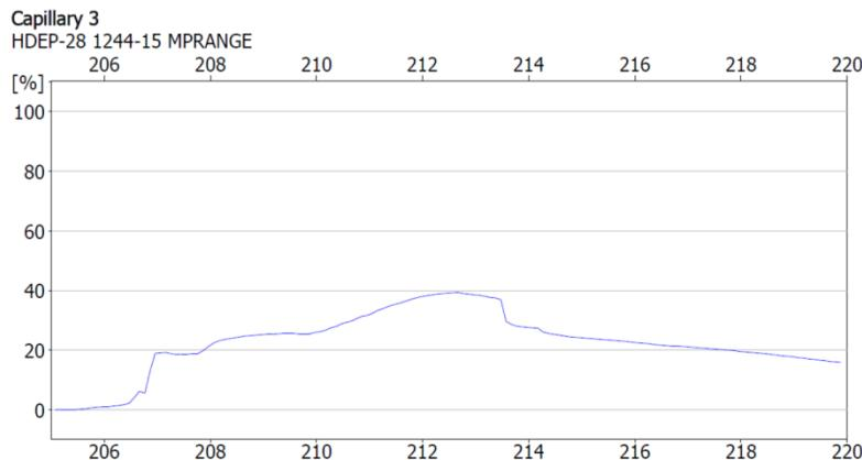
Figure 4: Melting curve for the sample purchased as HDEP-28.
