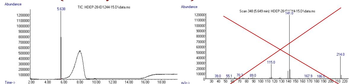
Chromatogram and MS obtained at our standard analytical conditions (inj. Port 280 st. C). Sharp and broad peak shows practically identical spectra. Both are missing of m/z = 84.
