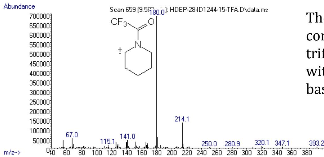
The obtained mass spectrum corresponds to trifluoroacetylderivative of HDEP-28, with molecular ion  $m/z$  939 and a base peak at  $m/z$  180.
