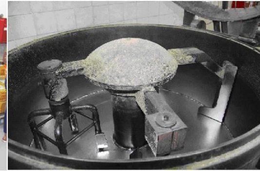
Mixing machine: raw plant material + synthetic cannabinoid dissolved in acetone is mixed until acetone is evaporated
