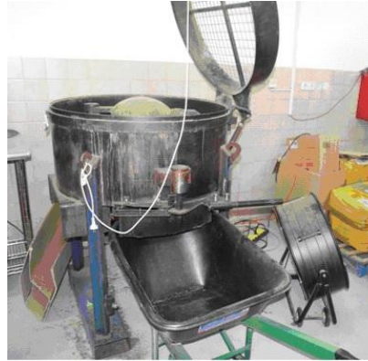
Mixing machine: raw plant material + synthetic cannabinoid dissolved in acetone is mixed until acetone is evaporated
