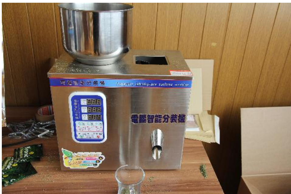
Figure 11: Machine for packaging herbal blends and bags for the Kronic product, found in production premises in Ljubljana
