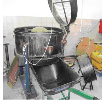
Mixing machine: raw plant material + synthetic cannabinoid dissolved in acetone is mixed until acetone is evaporated (some preparations can be sprayed with aromas and colourants can be added as well).
