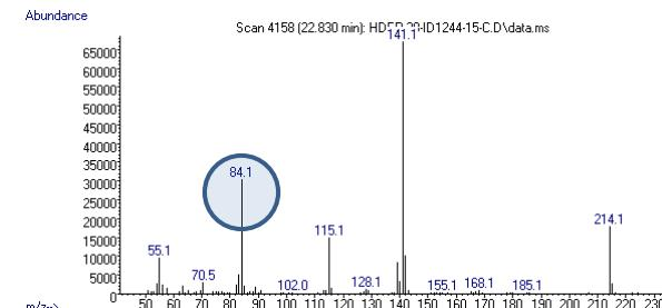
Chromatogram and MS obtained modified T(inj. Port 180 st. C, oven program changed as well)
